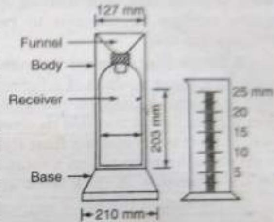
Fig. 31.4. Symon's non-recording type rain-gauge
