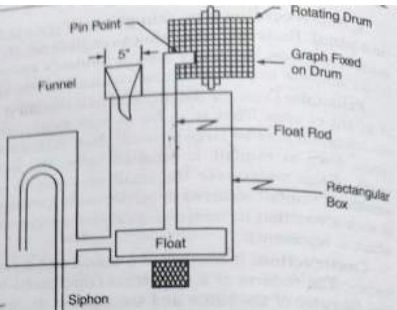
Fig. 31.5. Recording type rain-gauge
