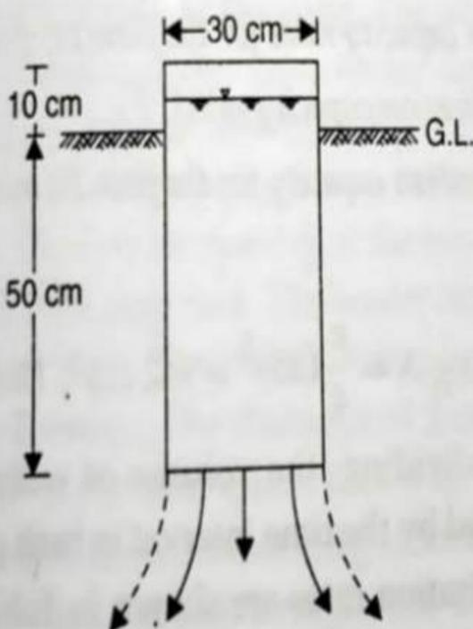
FIGURE 8.3 Tube infiltrometer.
