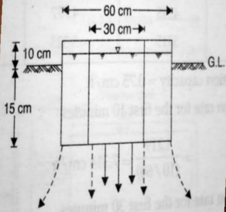
FIGURE 8.4 Double ring infiltrometers.
