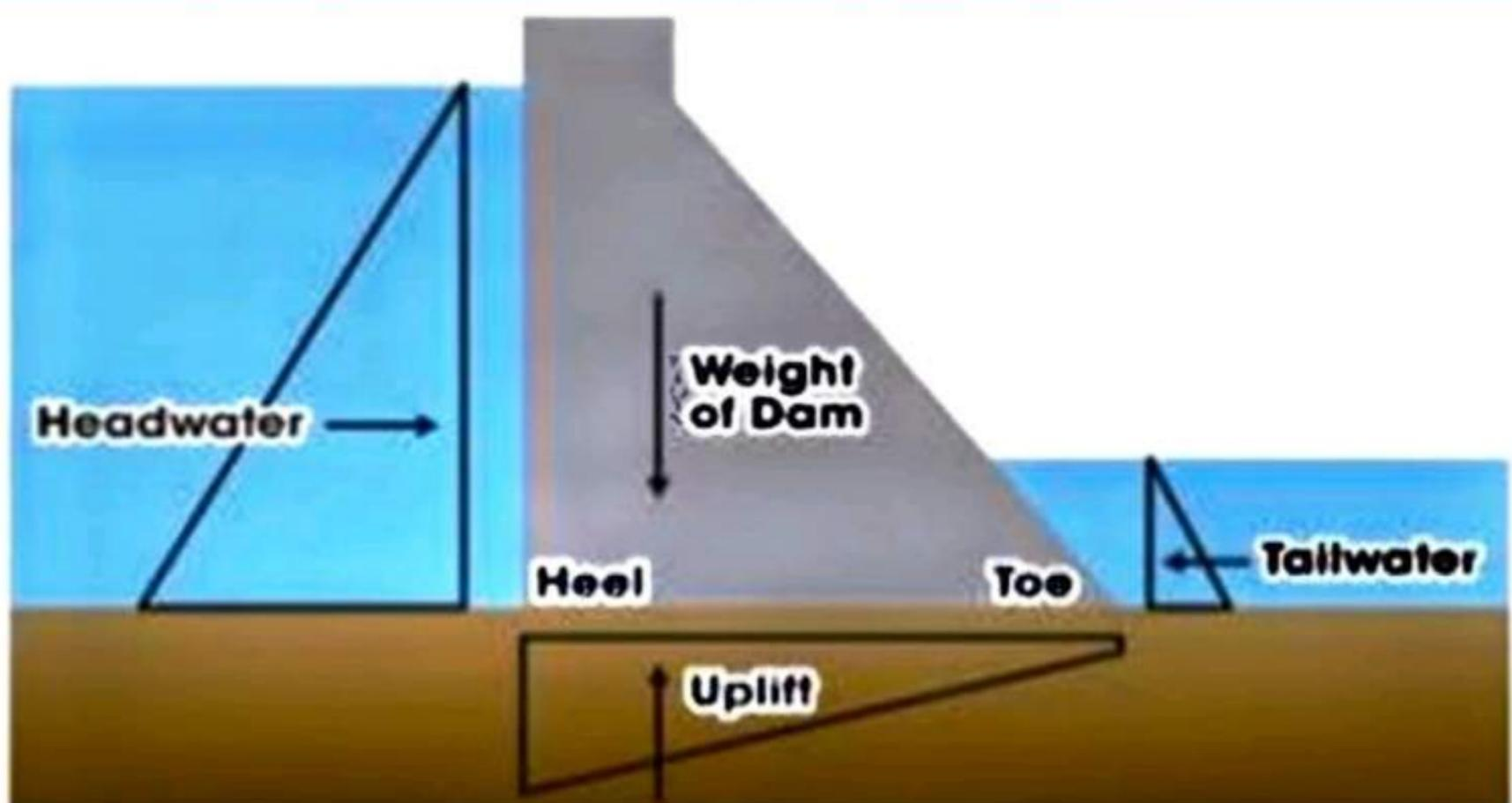
For any size of gravity dam, typical forces included in a two-dimensional stability analysis include headwater and tailwater, weight of the dam, and uplift.
