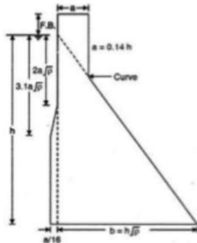
FIG. 8.19. PRACTICAL PROFILE OF A GRAVITY DAM.
