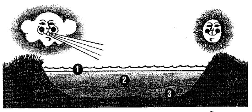
The top layer  $\mathbf{0}$  in a facultative lagoon is called the aerobic zone, the second layer  $\mathbf{2}$  is called the facultative zone, and the third layer  $\mathbf{3}$  is the anaerobic zone.
