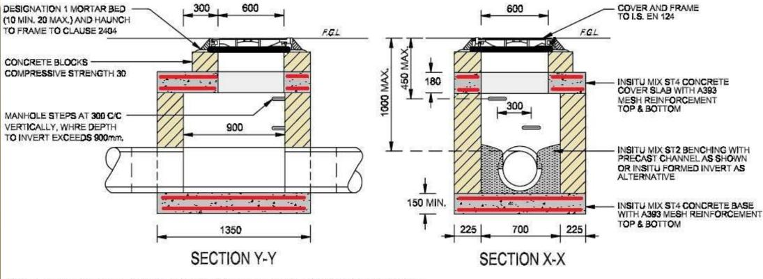
Constructing a typical shallow manhole 700x900mm
