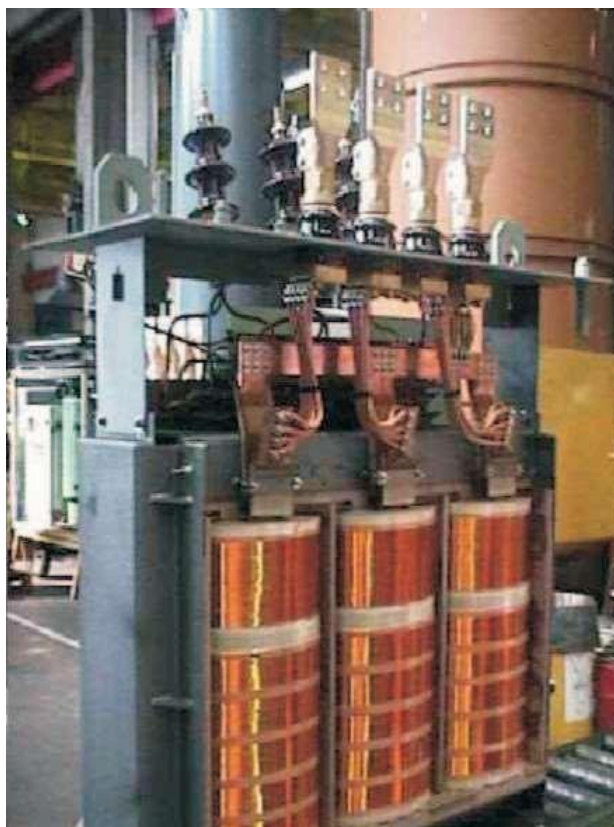
Figure 10.9 1600 kVA Amorphous Core Transformer
